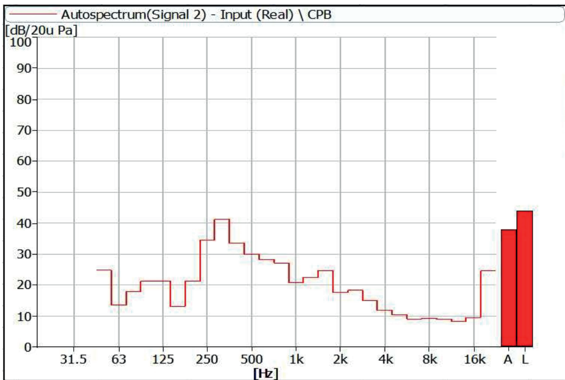
Figure 32 Noise Spectrum of Stage Luminaires (The Super Silence mode, Dynamic, No 2)
