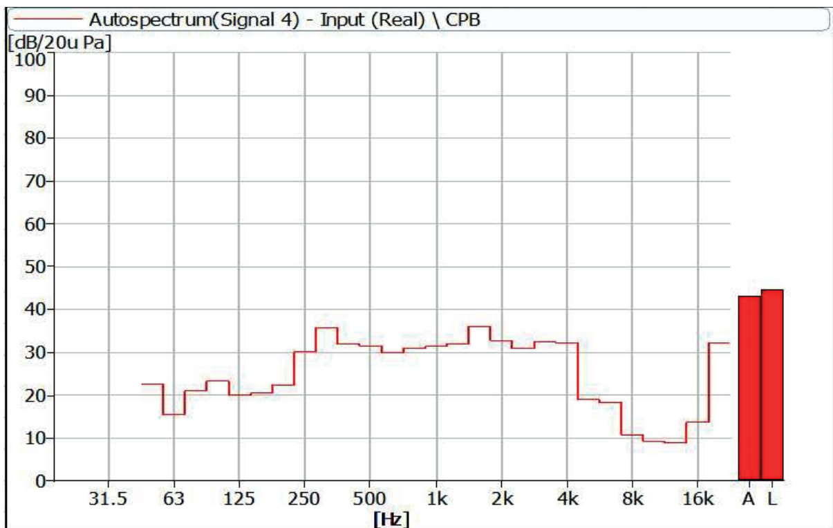
Figure 18 Noise Spectrum of Stage Luminaires (The Stage mode, Dynamic, No 4)
