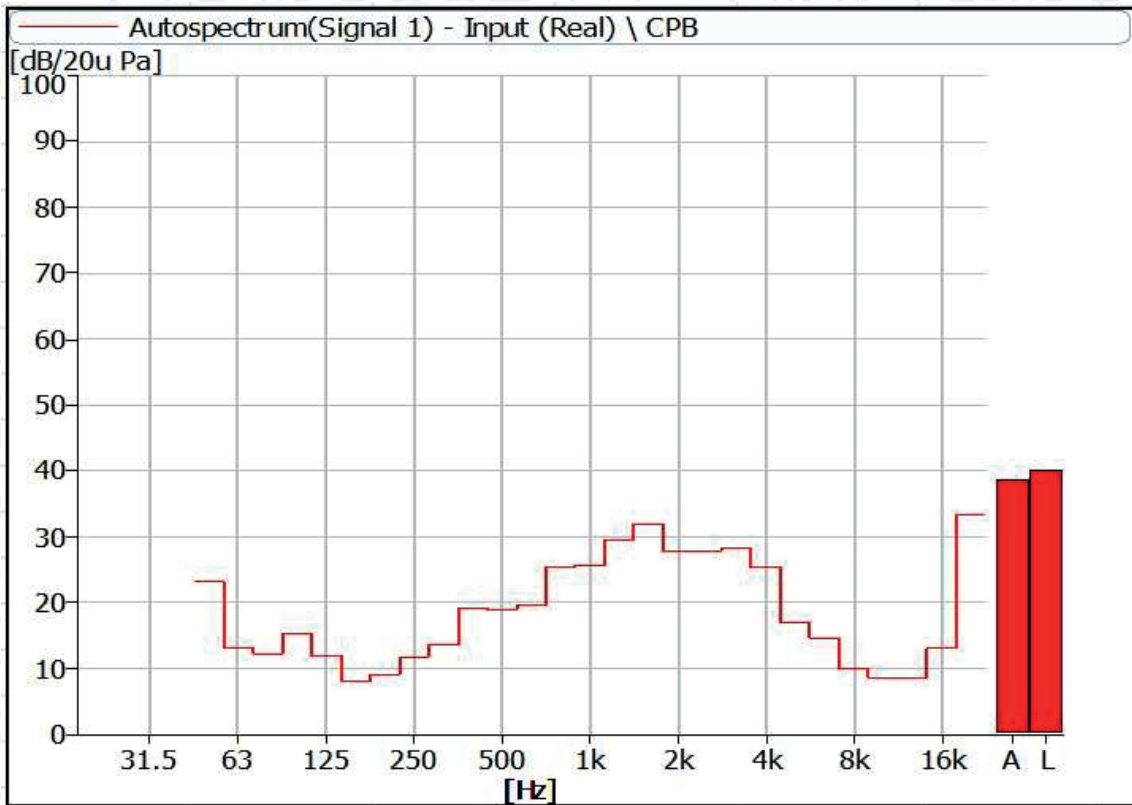
Figure 11 Noise Spectrum of Stage Luminaires (The Stage mode, Static, No 1)
