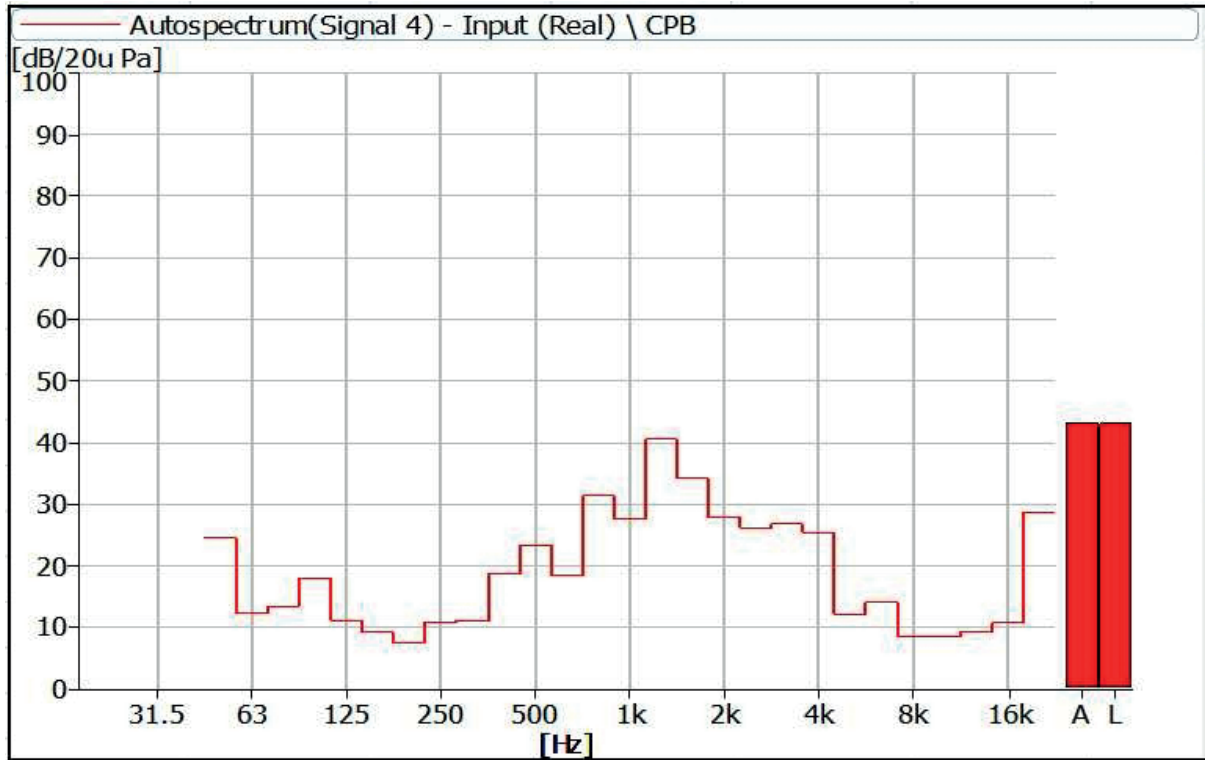
Figure 5 Noise Spectrum of Stage Luminaires (The Auto mode, Static, No 3)
