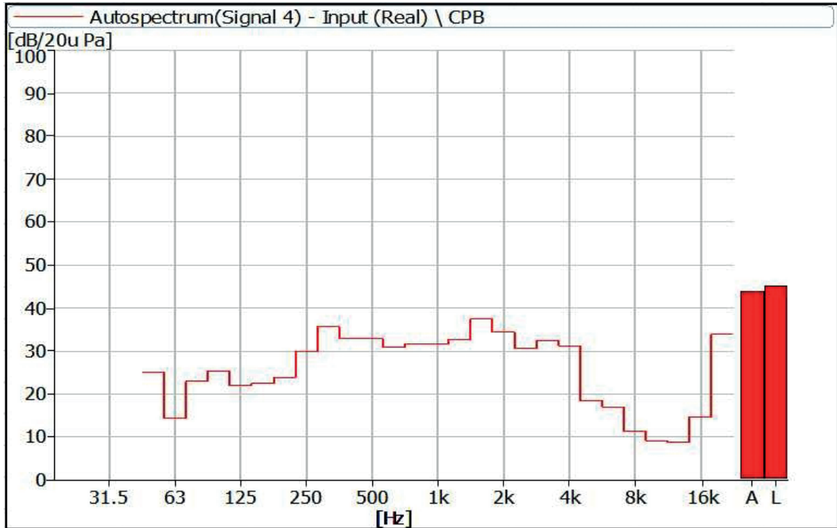
Figure 17 Noise Spectrum of Stage Luminaires (The Stage mode, Dynamic, No 3)
