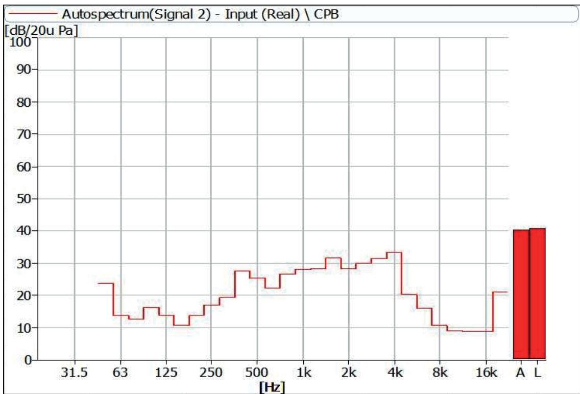
Figure 12 Noise Spectrum of Stage Luminaires (The Stage mode, Static, No 2)
