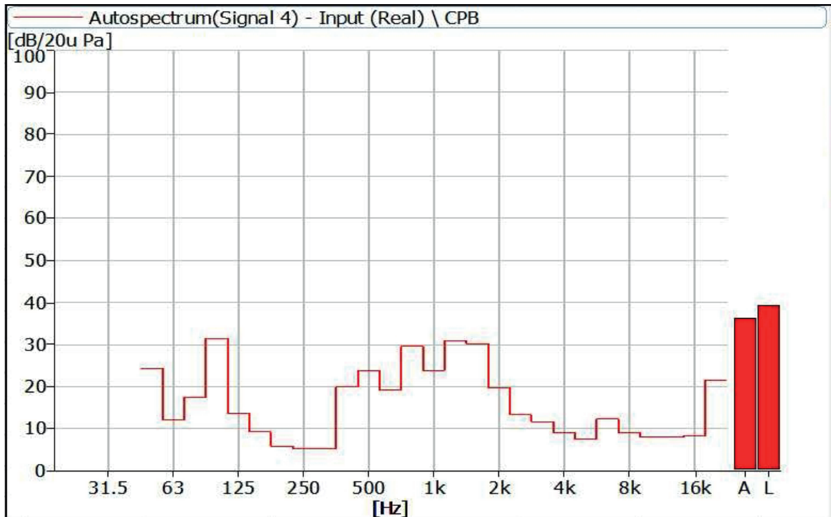
Figure 29 Noise Spectrum of Stage Luminaires (The Super Silence mode, Static, No 3)
