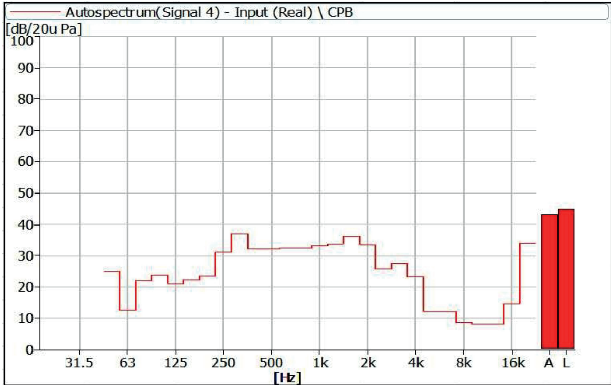
Figure 9 Noise Spectrum of Stage Luminaires (The Auto mode, Dynamic, No 3)
